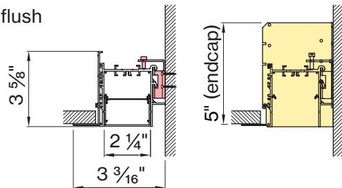
Fixture needs to be installed before ceiling is in place
